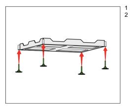
Place the plate stand at the desired installation location and align it.
