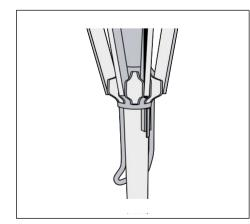
4 Press the sunshade roof onto the pole until the latch on the lower crown engages in the lock.
