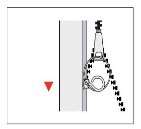
8 Loosen the eyebolt of the telescopic push rod in the key ring on the zip of the protective case.
