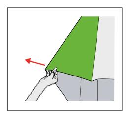
3 Pull the sunshade fabric out from between the struts to prevent it from becoming trapped or damaged.
