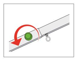
2 Open the knurled screw on the telescopic push rod.
